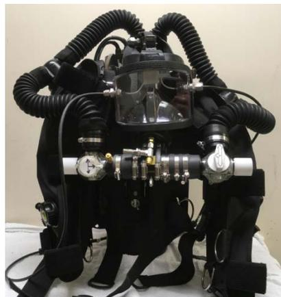
**Fig.1. Modified Megalodon rebreather.** Customized to accept gas from multiple sources and accommodate two forehead pulse oximeters.
