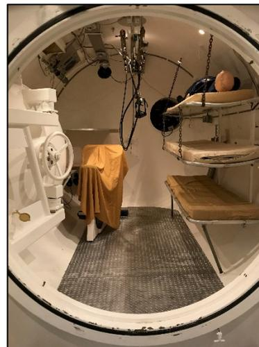
**Fig.1. DISSUB simulation chamber interior.** The chamber (23 ft. long and 9 ft. diameter) contains three racks for sleeping, mimicking the berthing facilities aboard a submarine.
