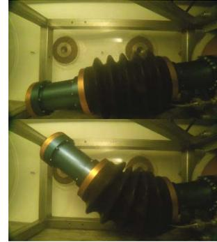
**Fig.3. Joint being tested at NSWCPCD, arm flexing up to ~55 degrees.**
