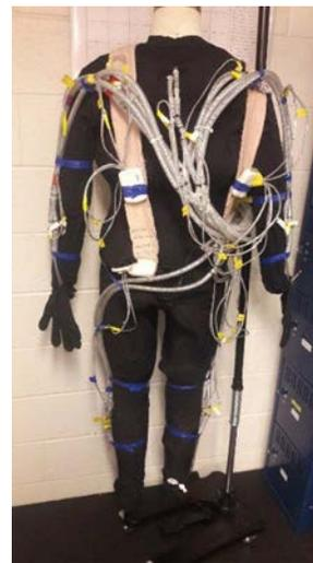
**Fig.2. Tubesuit with thermistors placed.** electrical tape holds tubing in place, bandage wrap is used for T-8 placement on back as well as tubesuit legs garment support..
