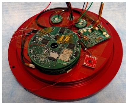
**Fig.1. DBD Testbed System.** This testbed system used electronics from QUASAR's dry electrode EEG headsets.
