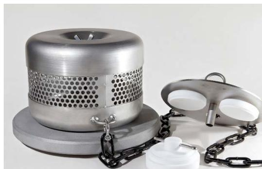
**Fig.1. ChemCatcher passive sampler.** One of the commercially available samplers to test for chemical contaminants. The contaminants must be selected in advance, and the sampler is then left underwater for an extended time period prior to retrieval and laboratory testing.
