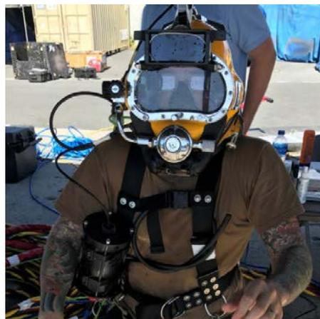
**Fig.4. DAVD Ph2 for KM37 Dive Helmet.** Navy diver ready to test the DAVD prototype configured for the US Navy KM37 helmet at MDSU-1 Joint Base Pearl Harbor.
